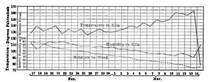
Fig. 99.—Typical conditions in a kiln during a run.
